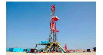
300 TON 330 TON DRILLMEC 27 1/2 INCH DRILLMEC MAS5000 1 1/4 INCH Top Drive TESCO 350 DRILLMEC 12T1600
